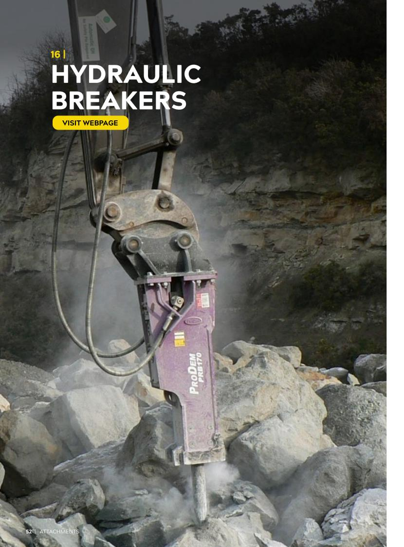
These powerful attachments are ideal for most types of demolition, landscaping and roadworks. We have breakers available for all excavator sizes from the smallest to the largest. They are perfect for rock breaking or breaking up large areas of reinforced concrete.
