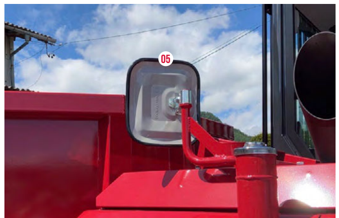
04 05 New mirror for reverse seat position to improve rear left lateral visibility
