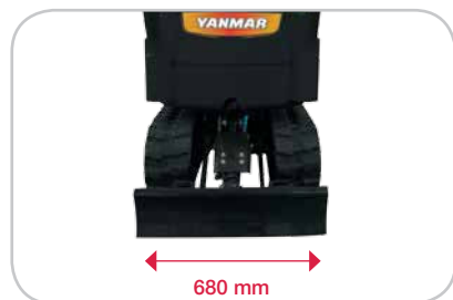
Retracted undercarriage to allow easier manoeuvre
