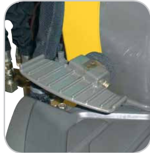
Retractable pedals (PTO pedal and swing control pedal)
