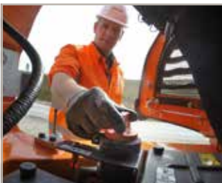
Battery cut-off switch
