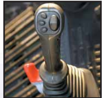
Joysticks with proportional control button for attachments
