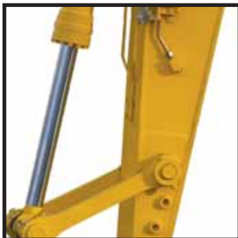
Quick-coupler piping standard
