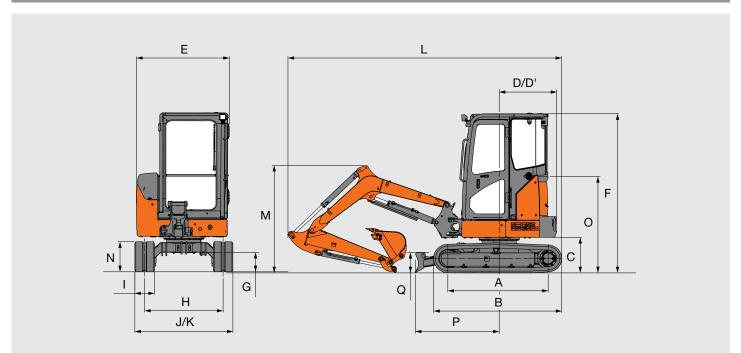
This illustration shows with 1.30 m arm, 0.080 m<sup>3</sup> bucket and 300 mm rubber shoes.
