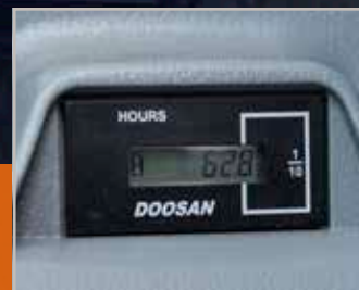
Hour meter (from ground level)
